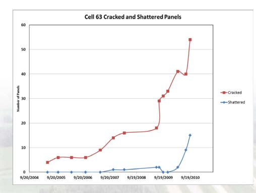
Figure 4. Development of cracking distress in Cell 63.
