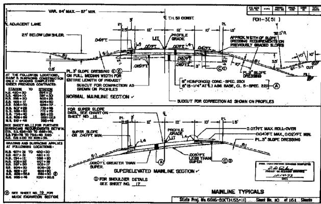
Figure 3.2. Mainline Typical Sections for 1972 TH 53 Project
