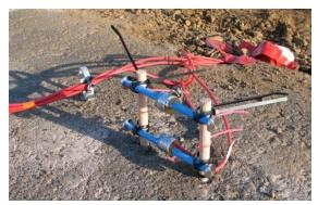
Figure 2.3. Dynamic Strain Sensors [Left] and Environmental Strain Sensors [Right]
