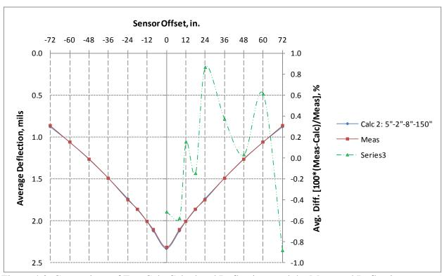
Figure 4.3. Comparison of EverCalc Calculated Deflections and the Measured Deflection
