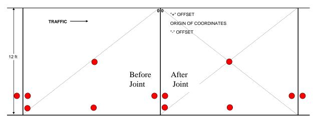
Figure 4.1. Routine FWD Testing Locations in Test Cell 53-1
