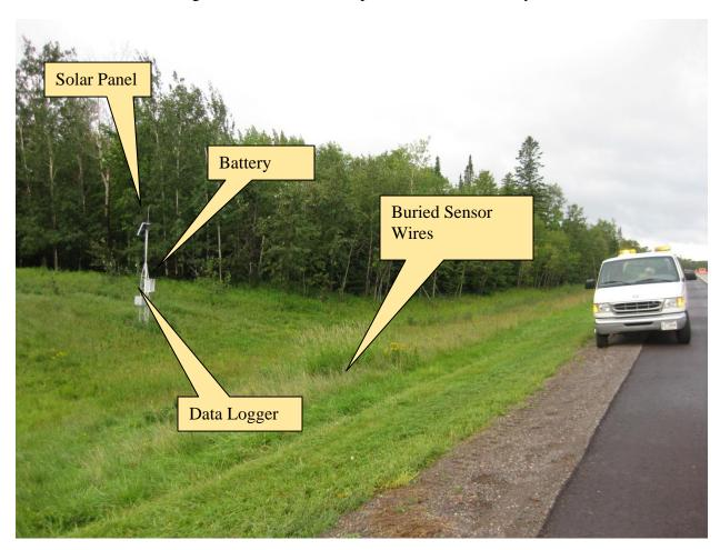
Figure 2.5. Completed Data Collection System
