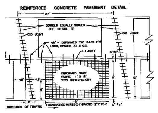
Figure 3.3. Reinforced Concrete Pavement Detail for 1972 TH 53 Project
