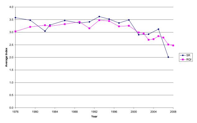
Figure 3.5. Average Pavement Condition Prior to Overlay
