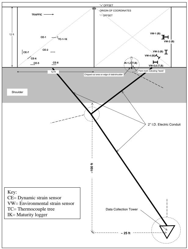
Figure 2.2. Cell 53-1 Instrumentation and Data Collection System Layout
