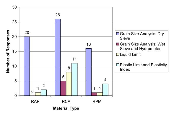
Figure 12: Specification Tests Used by Material Type
