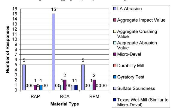
Figure 16: Aggregate Quality Tests for Toughness
