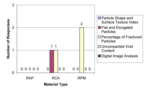
Figure 19: Aggregate Quality Tests for Particle Geometric Properties
