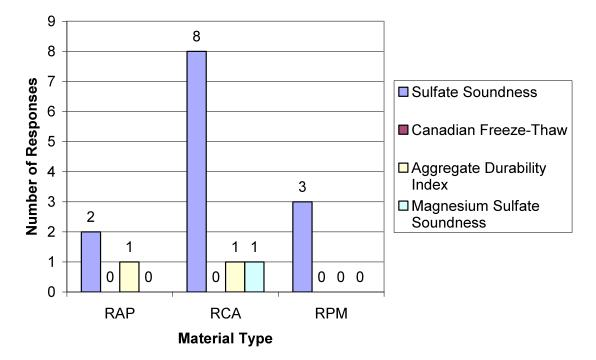
Figure 17: Aggregate Quality Tests for Durability
