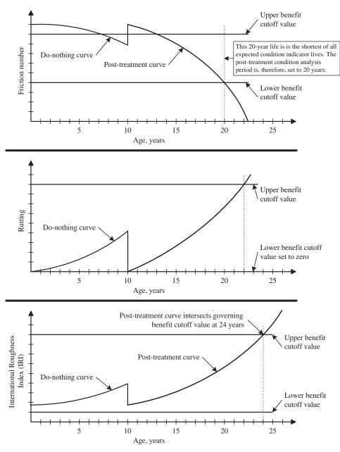
*Figure 6.* Determination of the overall post-treatment condition expected service life (analysis period).
