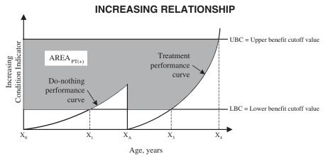
Note: for this case,  $X_2 = X_A$  as  $X_A$  is less than the projected intersection of the do-nothing curve and the LBC.
