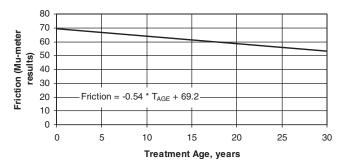
Figure 17. Assumed post-treatment seal coat friction relationship for Case Study 1—Arizona.
