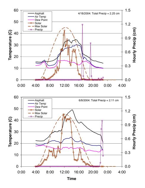
Figure 6.7. Measured pavement temperature and climate conditions for an event with a high cooling rate and a high heating rate
