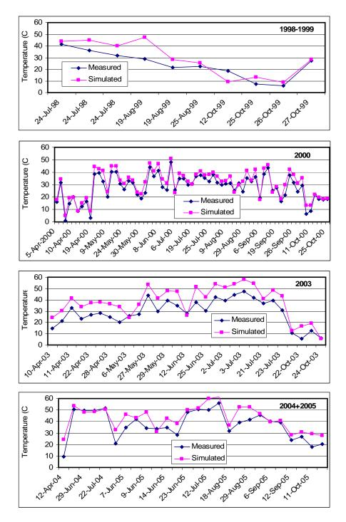
Figure 6.34. Measured vs. simulated pavement surface temperature for MnROAD test cell 35.
