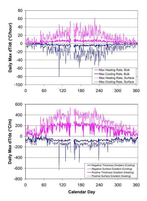
Figure 6.6. Daily extreme temperature gradient (dT/dz) and rate of change of temperature (dT/dt) for test cell 33, 2004.
