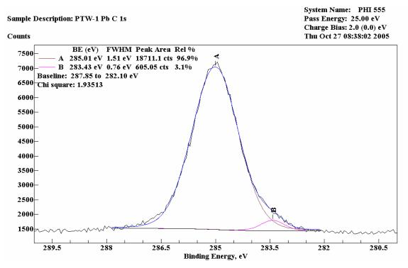
Figure 3.14. XPS testing results for specimen PTW-1 Pb
