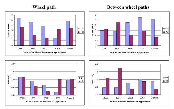
Figure D.21. Stress and strain at failure from DTT for upper layer, TH 56 1999 sections
