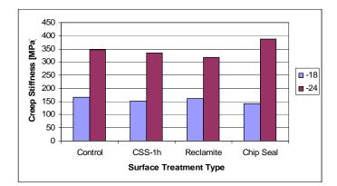
Figure 5.4. Stiffness at 60 sec. for wheel path, TH 251 sections
