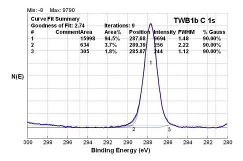
Figure 3.21. XPS testing results for specimen TWB1b
