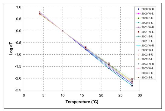
Figure 5.12. Log  $a_T$  vs. temperature for TH 56 1995 sections.
