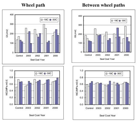
Figure D.52.  $G_f$  and  $K_{IC}$  for upper layer, TH 56 1999 sections
