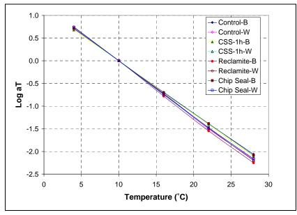
Figure 5.17. Log  $a_T$  vs. temperature for TH 251 sections.
