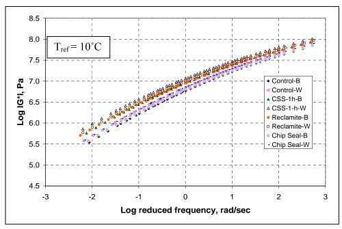
Figure 5.14. Complex modulus master curves for TH 251 sections.
