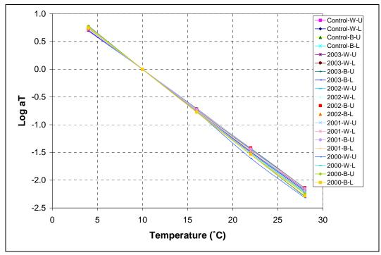
Figure 5.13. Log  $a_T$  vs. temperature for TH 56 1999 sections.
