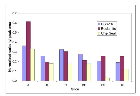
Figure 5.24. Carbonyl peak area for samples located in the wheel path in TH 251
