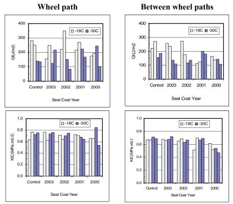
Figure D.53. G<sub>f</sub> and K<sub>IC</sub> for lower layer, TH 56 1999 sections
