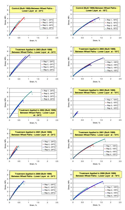
Figure D.18. DTT curves for between wheel paths, lower layer, TH 56 1999 sections
