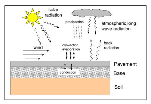
Figure 6.17. Schematic diagram of the processes considered in the pavement temperature model.
