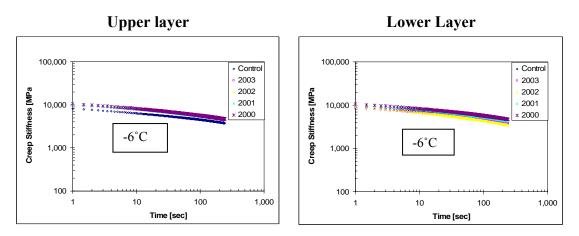
Figure D.39. Mixture creep stiffness vs. time for samples located in wheel path, TH 56 1999 sections
