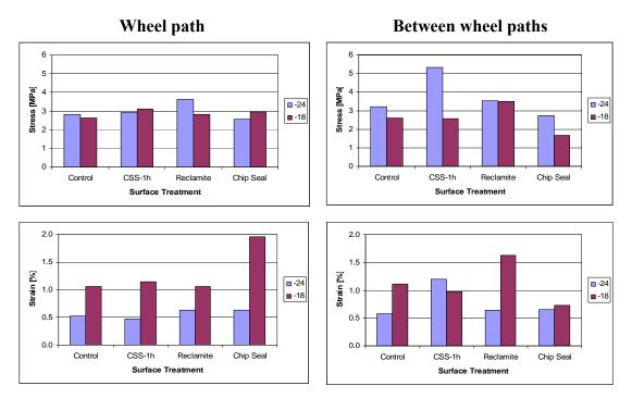
Figure D.25. Stress and strain at failure from DTT, TH 251
