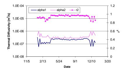
Figure 6.38. Thermal diffusivity (α<sub>1</sub> or α<sub>2</sub>) from 7-day running samples of 15-minute data, January 1 – December 31, 2002, MnROAD cell 33
