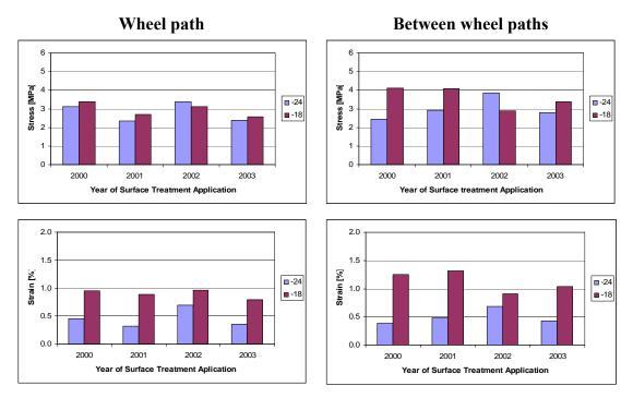
Figure D.19. Stress and strain at failure from DTT for upper layer, TH 56 1995 sections
