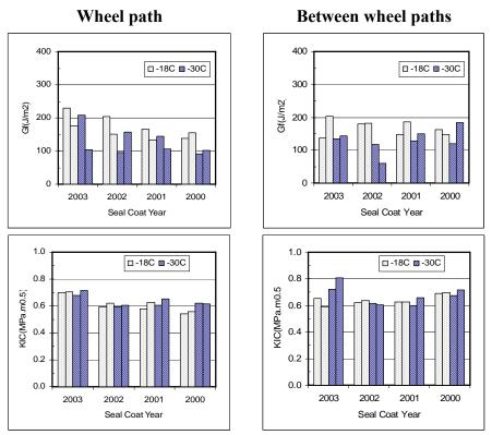
Figure D.50. G<sub>f</sub> and K<sub>IC</sub> for upper layer, TH 56 1995 sections
