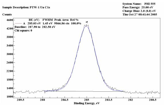
Figure 3.11. XPS testing results for specimen PTW-1 Ua
