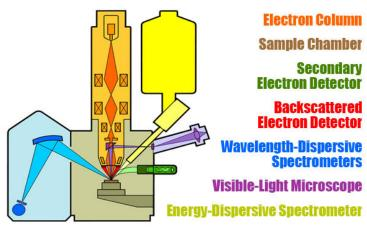
Figure 3.24. Electron microprobe components [21]
