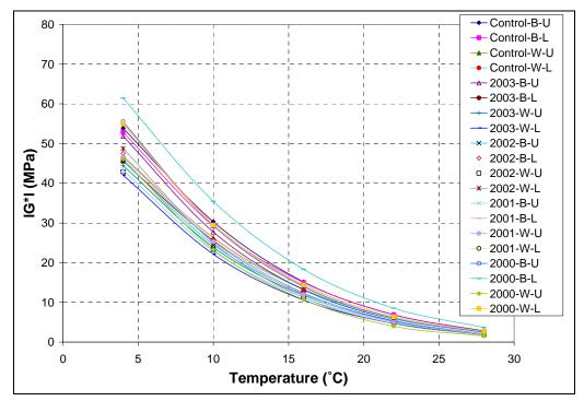
Figure 5.11. |G\*| at 10 rad/s vs. temperature for TH 56 1999 sections.
