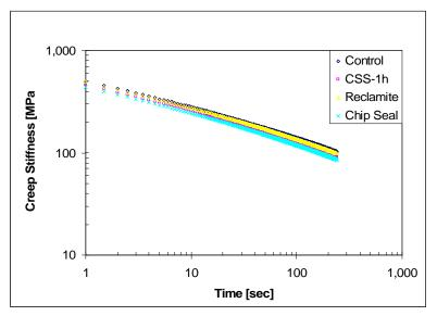
Figure 5.3. Creep stiffness vs. time for wheel path at -18°C, TH 251 sections
