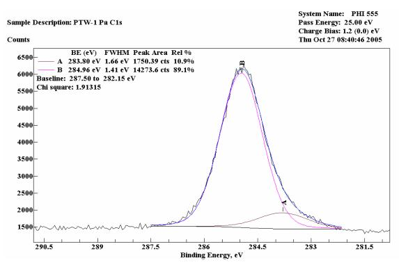
Figure 3.13. XPS testing results for specimen PTW-1 Pa
