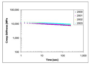
Figure 5.30. Mixture creep stiffness vs. time for between wheel paths, upper layer at -18°C, TH 56 1995 sections
