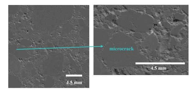
Figure 3.25. Electron microprobe images for laboratory prepared specimen
