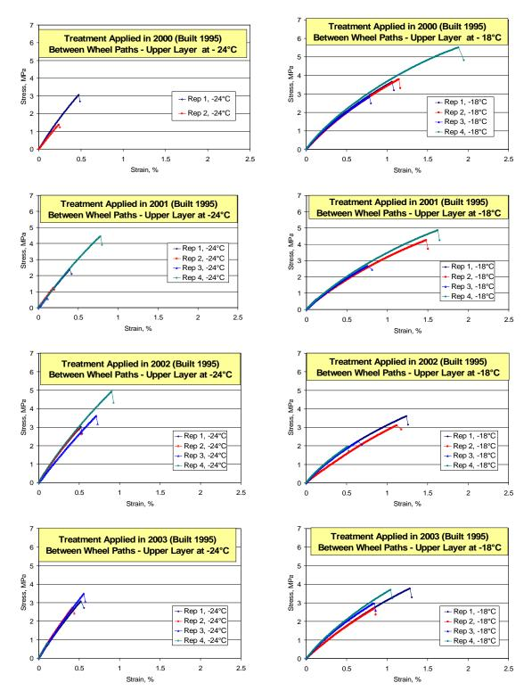
Figure D.13. DTT stress vs. strain curves for between wheel paths, upper layer, TH 56 1995 sections
