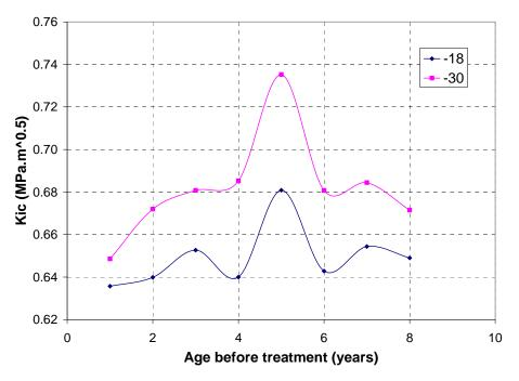
Figure 5.38. Average fracture toughness vs. age for TH 56 sections
