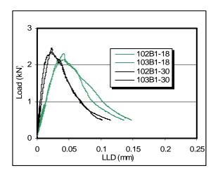
Figure 5.34. Load-LLD curves from SCB testing of control samples at -18°C and -30°C, between the wheel paths, TH 56 1999 sections
