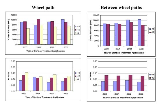
Figure D.40. Stiffness of the mixture and m at 60 sec. for upper layer, TH 56 1995 sections
