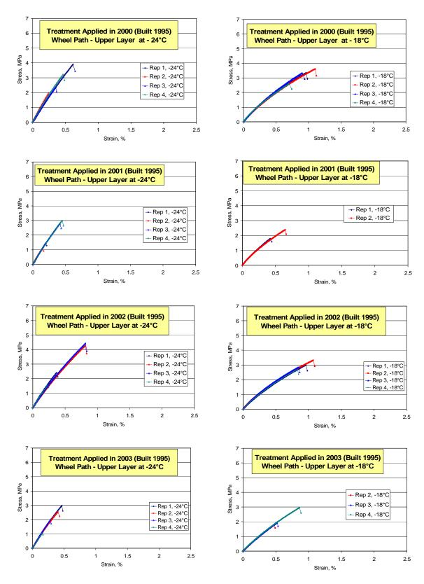
Figure D.11. DTT stress vs. strain curves for wheel path, upper layer, TH 56 1995 sections
