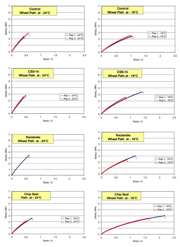
Figure D.23. DTT stress vs. strain curves for wheel path, TH 251
