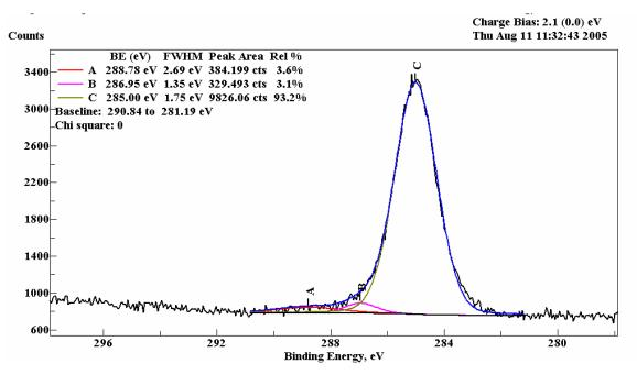
Figure 3.2. XPS testing results for specimen T-1
