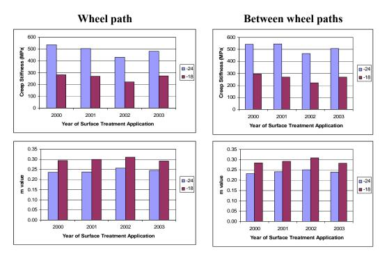
Figure D.5. Stiffness and m at 60 sec. for upper layer, TH 56 1995 sections
