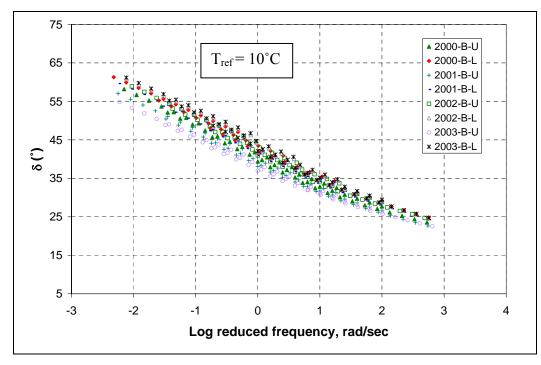
Figure D.29. Phase angle master curves for between wheel paths samples, TH 56 1995 sections
