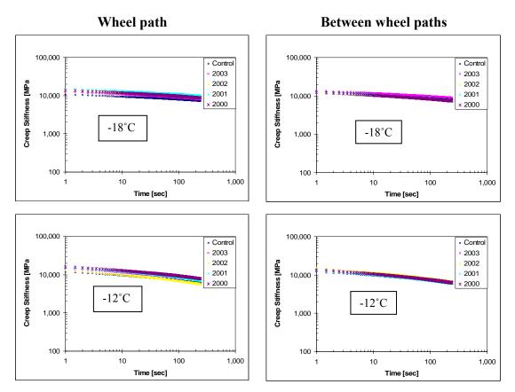
Figure D.38. Mixture creep stiffness vs. time for lower layer, TH 56 1999 sections
