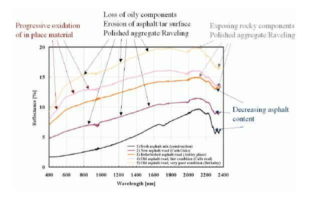
Figure 3.33. Spectra of different asphalt pavements taken from [29].
