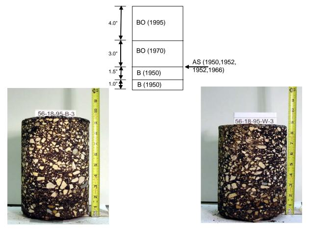
Figure A.8. Specimens from section 18, TH 56
