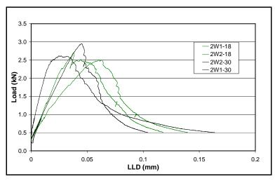
Figure 5.36. Load-LLD curves from SCB testing of control samples at -18°C and -30°C, wheel path, TH 251
