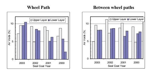
Figure 5.27. Air voids for samples from TH 56 1995 sections
