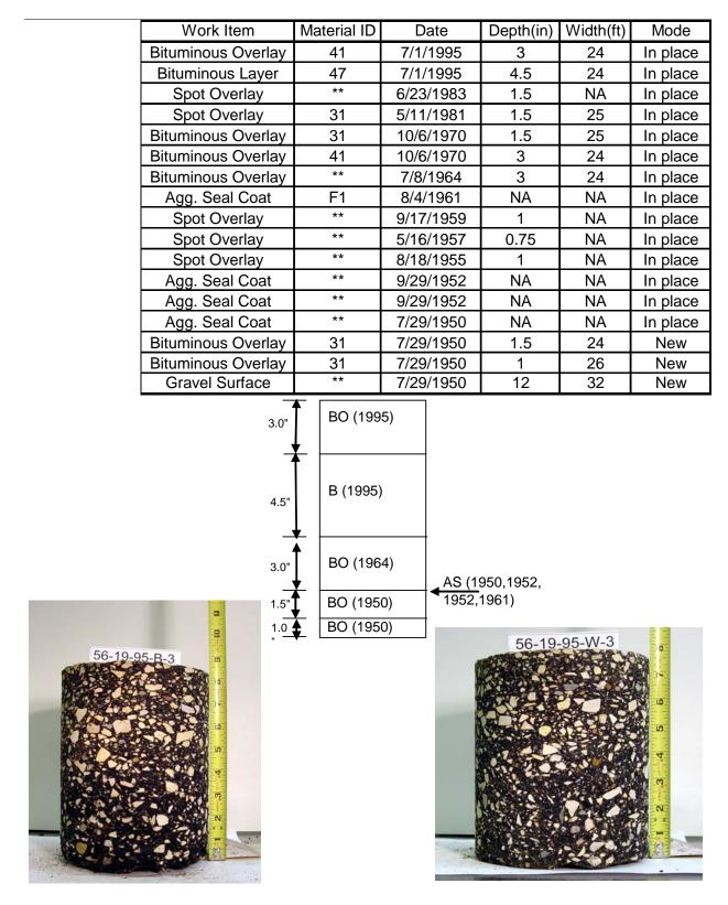
Figure A.9. Specimens from section 19, TH 56
