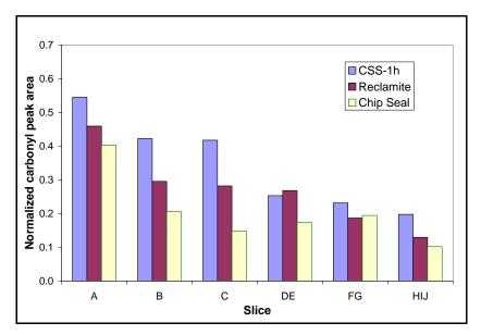
Figure 5.25. Carbonyl peak area for samples located between wheel paths in TH 251
