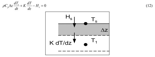
Figure 6.12. Schematic of surface heat transfer components
