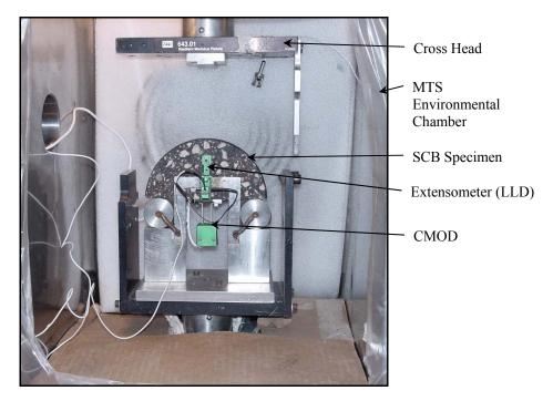
Figure 4.3. SCB test setup [39]
