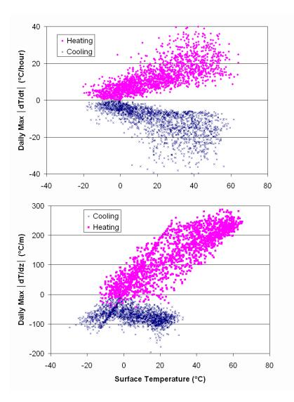
Figure 6.16. Daily extreme temperature gradient (dT/dz) and rate of change (dT/dt) surface temperature for test cell 33, Jan 1, 2001 – Dec 31, 2005.
