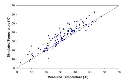
Figure 6.31. Measured vs. simulated pavement surface temperature for MnROAD test cell 34.
