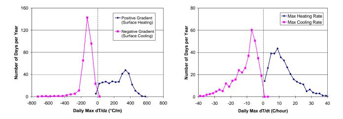
Figure 6.11. Distribution of daily extreme surface temperature gradient (dT/dz) and surface temperature rate of change (dT/dt) for test cell 33, 2001 – 2005. Each point represents an average yearly 2°C bin count for the five year period.
