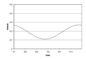
Figure 6.22. Calibrated seasonal variation of surface albedo for test cell 33, 2004. albedo =  $0.19+0.08*\cos(2\pi (cd+15)/365)$ , where cd is the calendar day.
