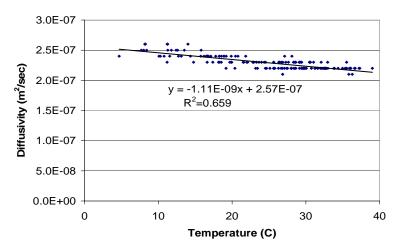
Figure 6.45. Thermal diffusivity versus weekly mean pavement temperature for MnROAD cell 33, week 11 through week 41, 2000-2005.
