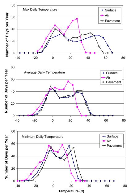
Figure 6.8. Distribution of daily maximum, minimum and average air, surface and pavement temperature for test cell 33, 2001 – 2005.
