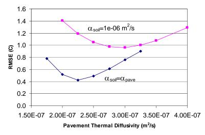
Figure 6.47. RMSE of simulated pavement temperature versus pavement thermal diffusivity for a fixed and a variable value of subgrade/soil diffusivity ( $\alpha_{soil}$ ).
