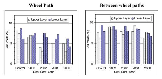
Figure 5.28. Air voids for samples from TH 56 1999 sections
