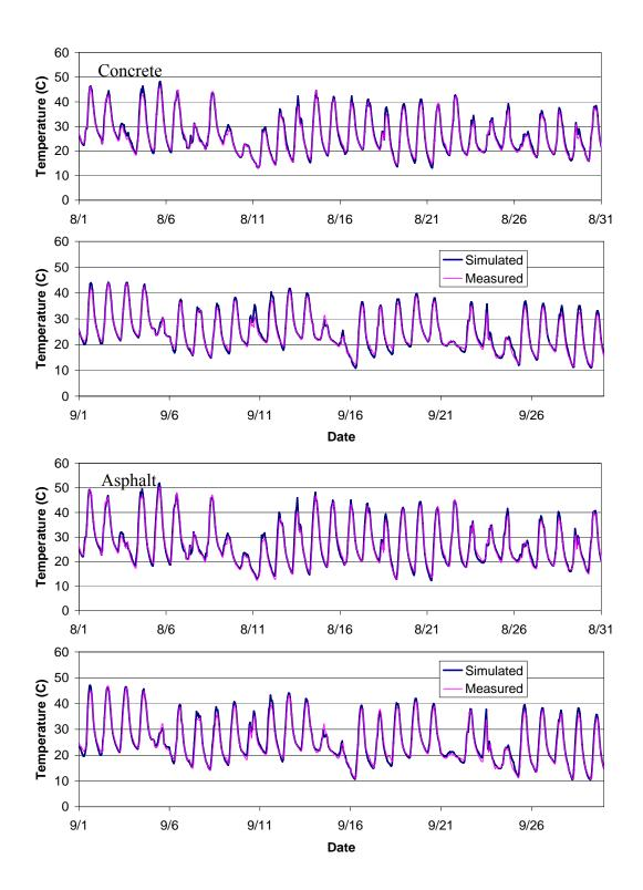
Figure 6.19. Simulated and measured pavement temperature (2.5 cm depth) for August and September, 2004, MnROAD test cells 33 (asphalt) and 38 (concrete), 1 hour time step.
