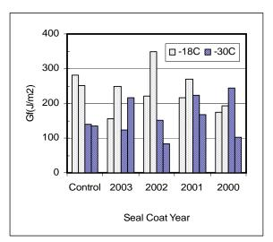
Figure 5.35. Fracture energy for samples in the wheel path, lower layer, TH 56 1999 sections
