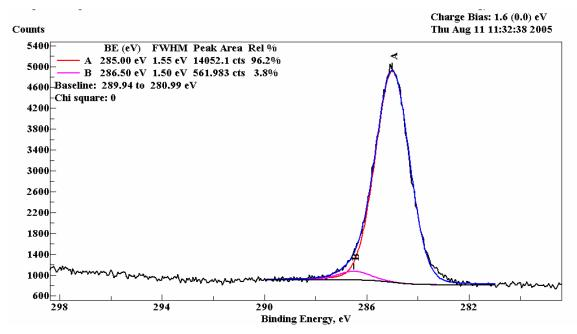
Figure 3.4. XPS testing results for specimen C-1
