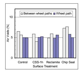
Figure 5.29. Air voids for samples from TH 251 sections
