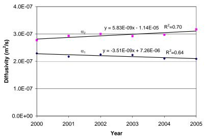
Figure 6.41. Thermal diffusivity (annual average) for MnROAD cell 33
