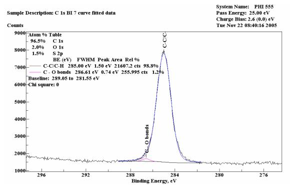
Figure 3.15. XPS testing results for specimen BI-7 Pa
