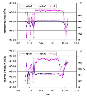
Figure 6.40. Thermal diffusivity in a sand/gravel subgrade layer (upper panel) and a clay base layer (lower panel), MnROAD cell 33
