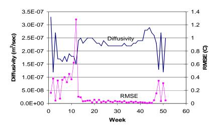
Figure 6.44. Thermal diffusivity and RMSE of fitted temperature versus week number for MnROAD cell 33, 2002.
