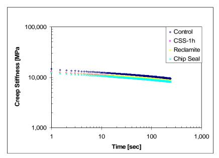
Figure 5.32. Mixture creep stiffness vs. time for wheel path at -18°C, TH 251 sections
