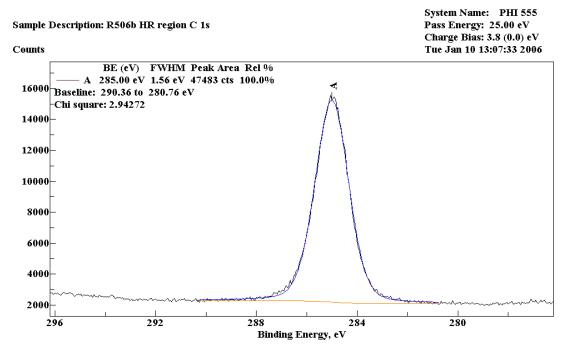
Figure 3.17. XPS testing results for specimen R506b
