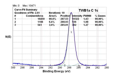
Figure 3.20. XPS testing results for specimen TWB1a
