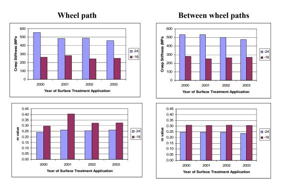
Figure D.6. Stiffness and m at 60 sec. for lower layer, TH 56 1995 sections
