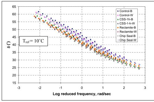
Figure 5.15. Phase angle master curves for TH 251 sections.
