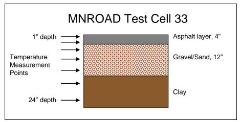
Figure 6.2. Schematic cross section of MnROAD test cell 33.
