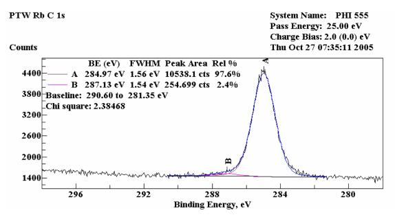
Figure 3.12. XPS testing results for specimen PTW-1 Rb
