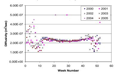
Figure 6.46. Thermal diffusivity versus week for MnROAD cell 33.
