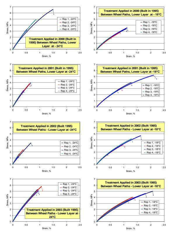
Figure D.14. DTT stress vs. strain curves for between wheel paths, lower layer, TH 56 1995 sections
