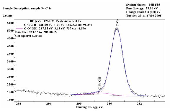
Figure 3.8. XPS testing results for specimen 34
