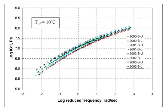
Figure D.28. Complex modulus master curves for between wheel paths samples, TH 56 1995 sections
