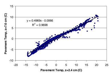
Figure 6.37. Measured temperature at 7.6 cm depth versus 2.4 cm depth in MnROAD cell 33, July 1 – July 8, 2002.
