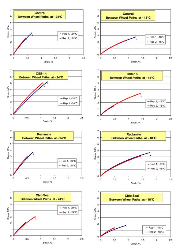
Figure D.24. DTT stress vs. strain curves for between wheel paths, TH 251
