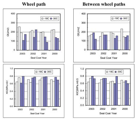
Figure D.51. G<sub>f</sub> and K<sub>IC</sub> for lower layer, TH 56 1995 sections
