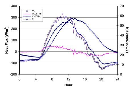
Figure 6.14. Variation of simulated surface temperature (Ts), surface heat flux (Hs), unsteady temperature change ( $\rho C_p dT_s/dt$ ), and vertical heat flux (KdT/dz) over 1 day (June 29, 2004).
