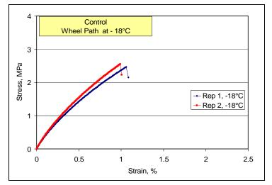
Figure 5.7. DTT stress vs. strain curve at -18°C for control, TH 251
