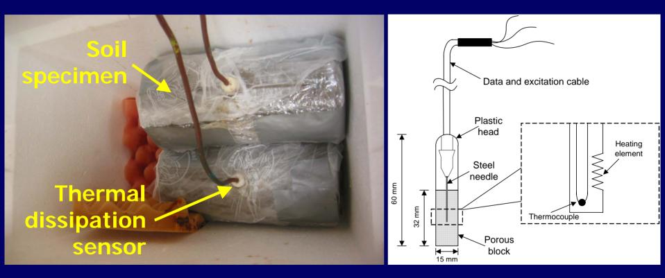
Schematic of Thermal Dissipation Sensor – Model 229 by Campbell Scientific Inc.
