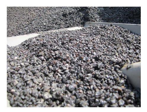
Figure 2 – Pre-coated stone used for entire project
