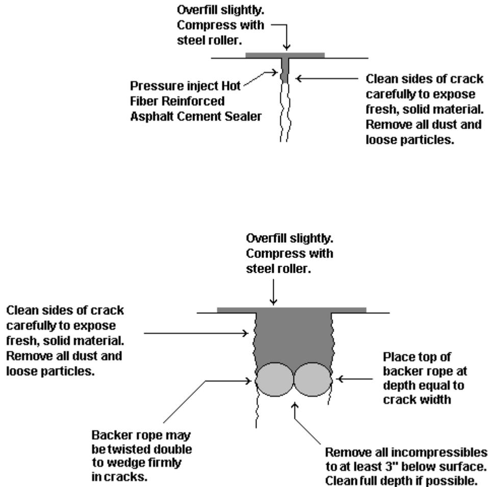
Figure 3. Overband sealing.
