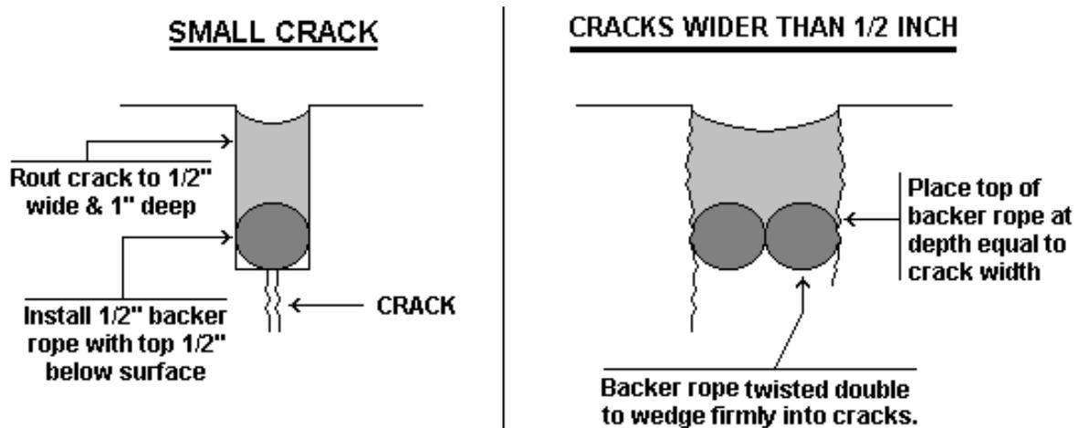
Figure 2. Crack sealing.
