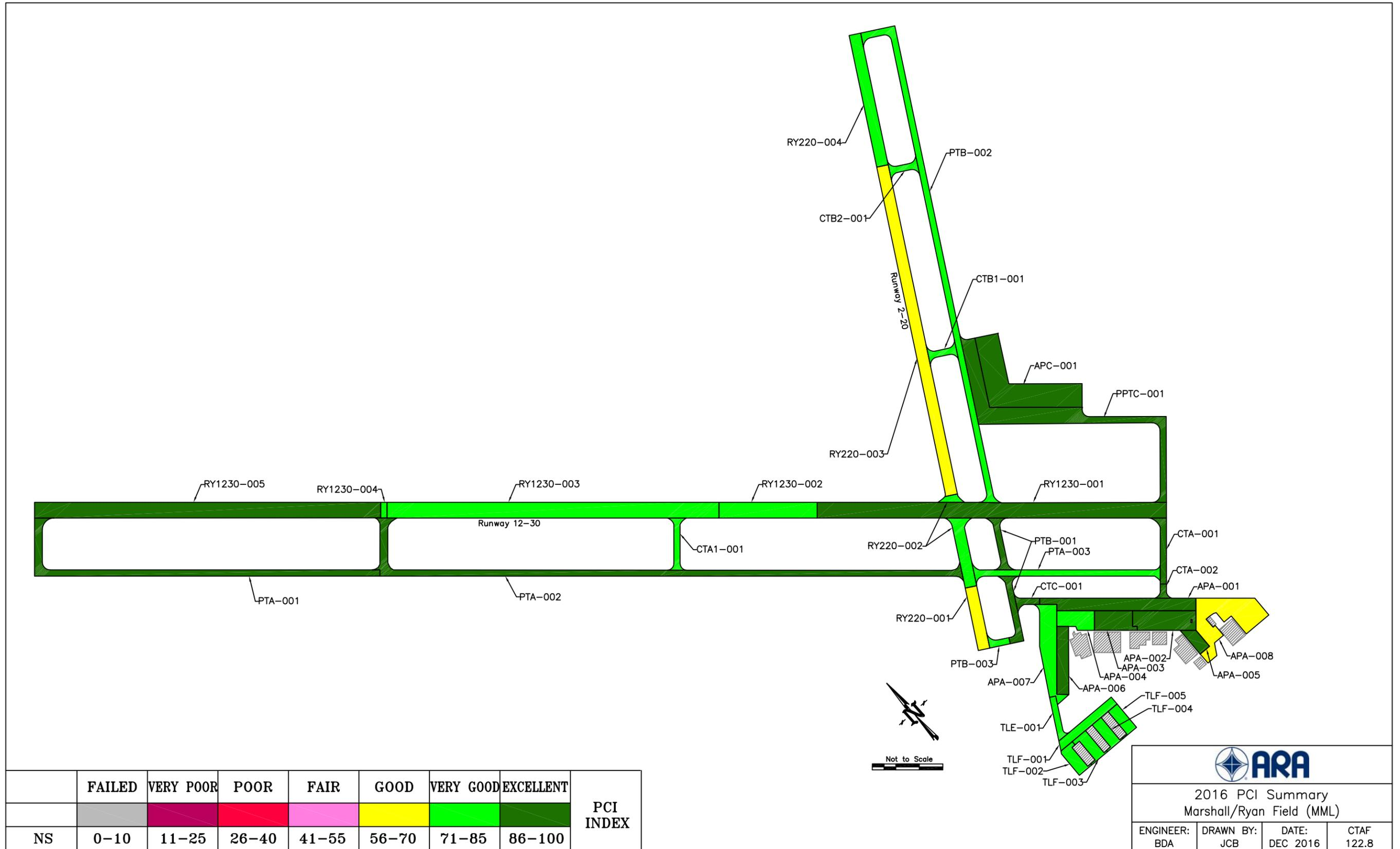
Figure 4. 2016 Pavement Condition Index Rating at Southwest Minnesota Regional Airport – Marshall/Ryan Field (MML).
