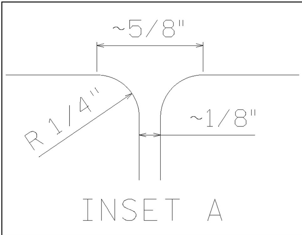
Figure 10b - Spec 2521.3c (allowable joint displacement)
