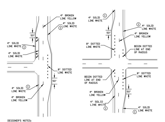
NO PASSING ZONE STRIPING IS OPTIONAL AT THE DISCRETION OF THE DISTRICT TRAFFIC ENGINEER FOR RURAL INTERSECTIONS NO PASSING ZONES AT INTERSECTIONS SHALL BE STRIPED FOR 500 FT ON BOTH SIDES OF THE INTERSECTION IF IT IS LOCATED WITHIN THE CITY LIMITS. NO PASSING ZONES AT INTERSECTIONS SHALL BE STRIPED IF LOCATED WITHIN ANY NO PASSING ZONE.
