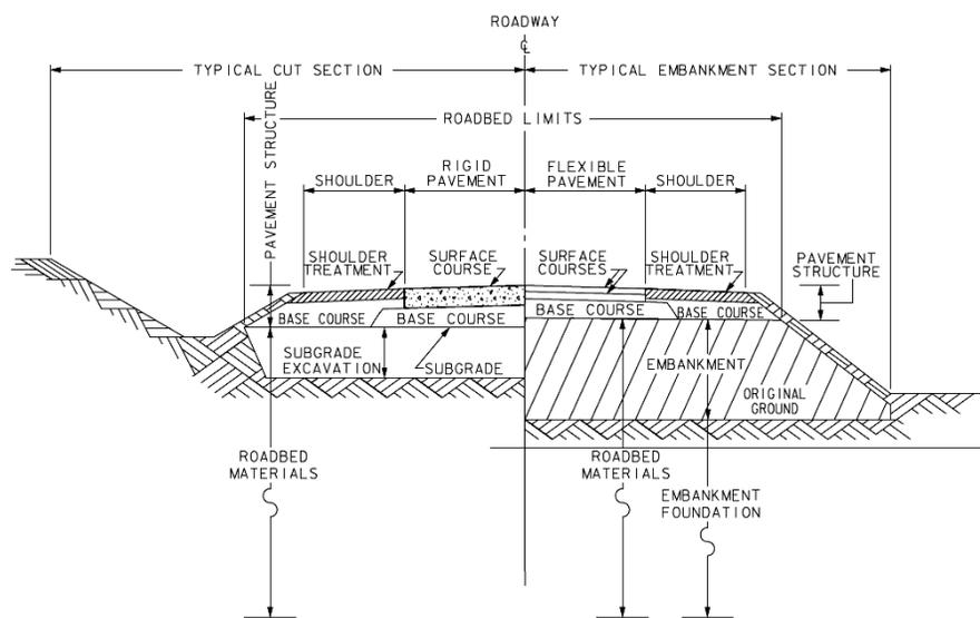
Figure 1: Typical Roadway Cross Section (Rural Section Shown)
