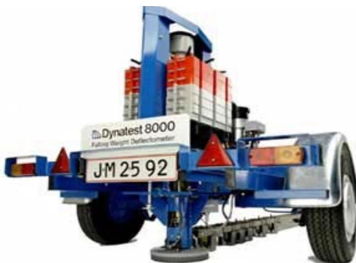
Roadway deflection under a load can be used as a measure of the load carrying capacity of a roadway. One tool that is currently used to measure this deflection is the Falling Weight Deflectometer (See [Figure 2](#)).
