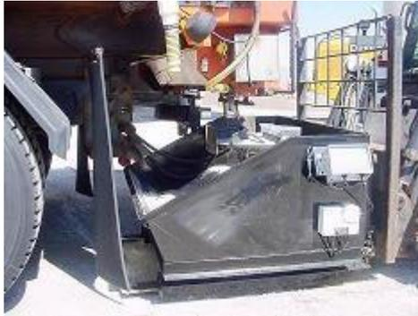
17. Press the Standby button to stop the AUGER
