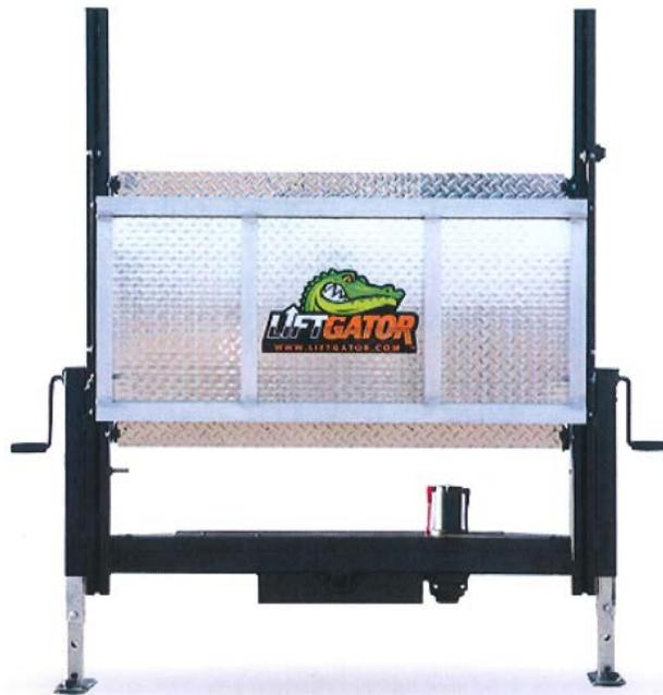
The LiftGator project was submitted by Brad Peterson in District 6W. The purpose of this lift-gate is to ease the lifting of equipment in and out of the truck bed. It is a self-contained unit that can be moved from truck to truck very easily.
