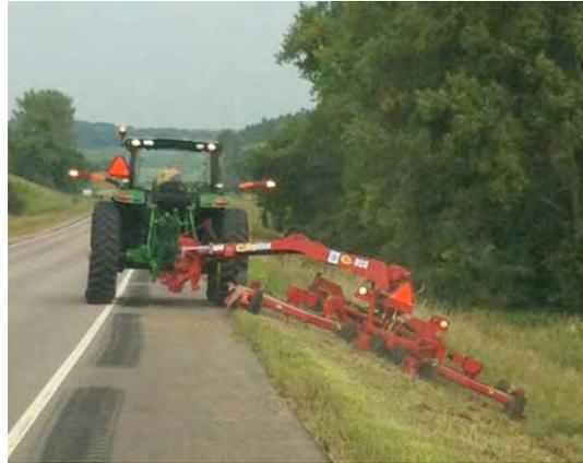
**Project Description:** The district is testing the Highline radial contouring hitch (RCH) batwing mower with a pivoting contouring hitch and walking caster wheels to mow roadside ditches. A typical hitch mower requires the tractor to leave the roadway to mow ditches and cannot reach the wet areas that the RCH batwing mower can reach by shifting the mower as needed while the tractor stays on dry ground.
