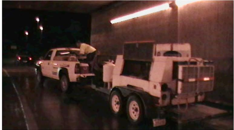
**Project Description:** Soda blasting is a new paint stripping technology that uses compressed air to propel a bicarbonate of soda-based media onto the surface to be cleaned or stripped.
