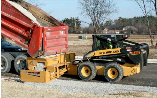
**Project Description:** Small repairs to gravel shoulders are currently made using sander conveyors on the rear of dump trucks. When a load of gravel has been emptied, the truck must leave the repair site to get a new load, which creates downtime if the material is far from the repair site. The district is testing a shoulder widening unit that is powered by a skid-steer tractor, which allows crews to use several trucks to feed the unit.
