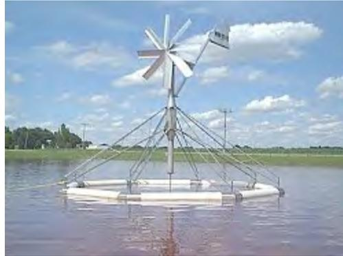
**Project Description:** Blowing snow is a concern on the Interstate 35 bridge over Albert Lea Lake. This project will use a wind-driven aeration system to maintain open water on the lake during the winter, which is expected to capture a significant amount of the blowing snow.
