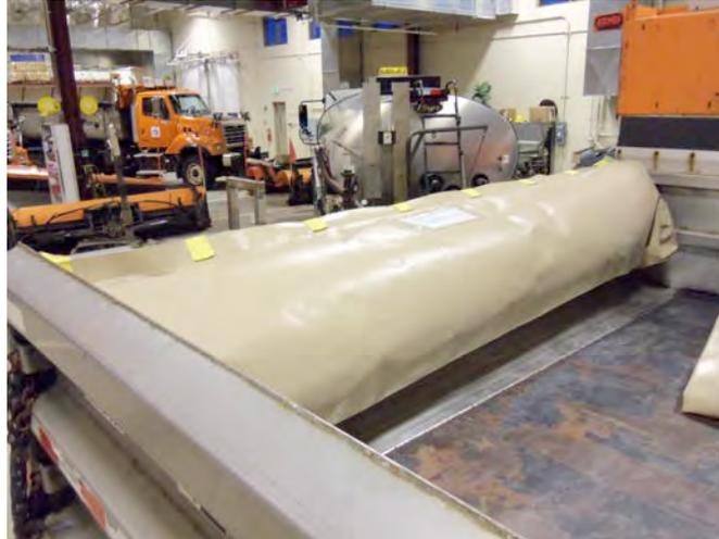
**Project Description:** MnDOT has traditionally used molded tanks to dispense liquid material during snow and ice operations. These tanks are cumbersome to maneuver and require a pump or pressure system to operate. As a potentially more flexible, cheaper alternative, District 7 wanted to test the effectiveness of brine bags. These bags hang from hooks by D rings and use a gravity flow system pressurized by the granular material in the box to supply a spray bar mounted in the sander.
