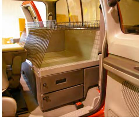
**Project Description:** The back seats of supervisors' pickups can be packed full of supplies, equipment and paperwork. These unsecured objects can be unsafe in the event of an accident and pose a security issue if valuables are in full view of potential thieves. The TruckOffice storage unit organizes paperwork, files and technical data, provides safe, secure laptop storage, and comes with an optional power inverter that can help with the use of electronics and other instruments in the field.
