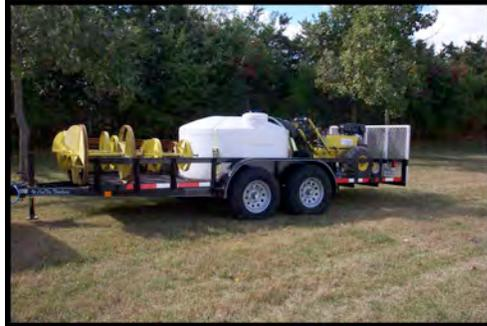
**Project Description:** The Rota-JETTER is a culvert cleaning machine that cleans culverts from 8 inches to over 36 inches in diameter. The machine's tools, cutting heads, water tank, and 110 feet of cleaning rods are mounted on a trailer; more cleaning rods can be added, up to 200 feet. Tools for smaller culverts are available, and the machine can be used to make horizontal bores of 8 feet or less.
