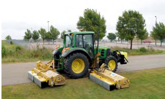
**Project Description:** In right of way maintenance, mowing is an expensive and labor-intensive operation. For many years, roadside maintenance programs have used herbicides in an effort to extend the mowing cycle. A wet cut mowing system creates efficiencies by combining the operations of a right of way mower and a chemical applicator for applying chemicals such as herbicides to stubble remaining after the mowing operation has been performed.
