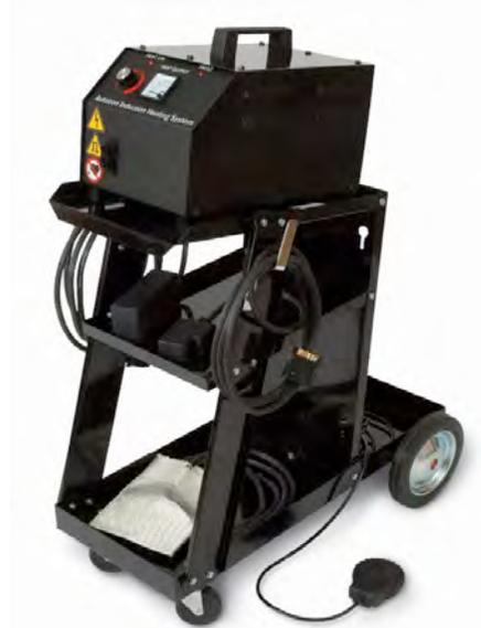
**Project Description:** The Autotron 3300 is an induction heating system that supports automobile repair operations. Using the Frame Pro Inductor attachment, workers can heat automobile frame rails and structural panels rapidly for straightening and relieving stress. The heat is very focused, easily monitored and controlled by the handheld inductor, and is safer than a torch flame for nearby heat-sensitive materials. The inductor can heat ¼-inch steel to 1300 F in just a few seconds.
