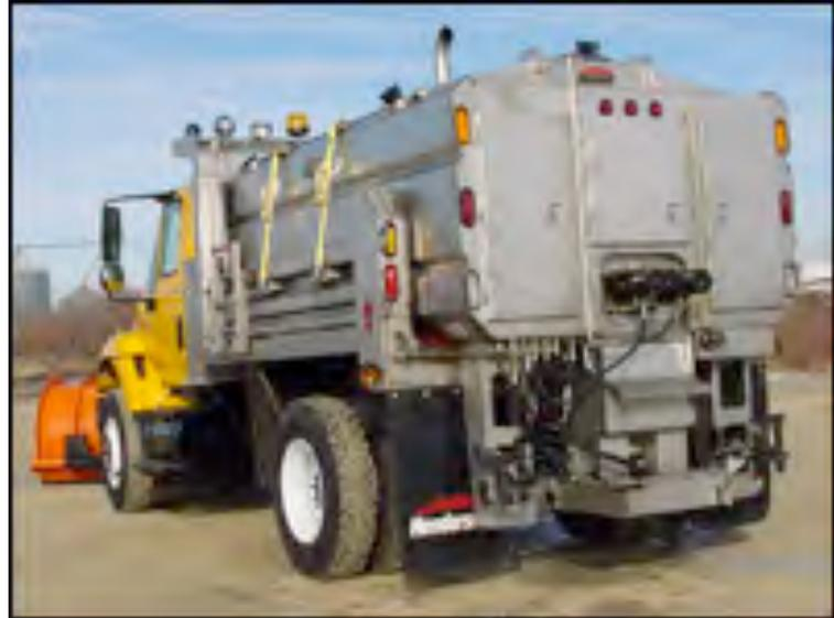
**Project Description:** Metro staff currently use a dump box with the tow plow to distribute granular materials on the roadway. However, only a quarter of the material in the box can be used because the tongue of the tow plow prevents raising the box to move material to the spreader. The First Response System is designed to work effectively with a tow plow fleet because it can discharge material in front of the box instead in the rear.
