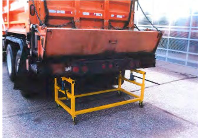
**Project Description:** Conveyors that spread material are typically installed on a truck with the use of a loader or skid loader outfitted with forks. In an effort to improve safety, increase efficiency and protect equipment from damage, district staff designed and constructed a conveyor stand as an alternative to the use of skid loaders for conveyor installation and removal.
