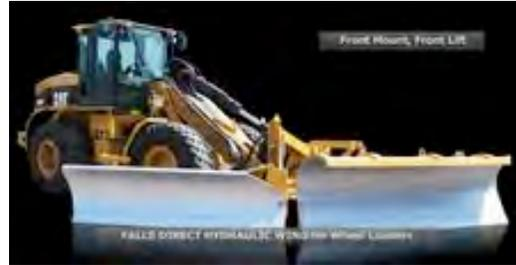
**Project Description:** The district will test a Universal reversible snowplow and wing assembly for use with its Case 721D front-end loader. The system includes the snowplow, wing and two mounting frames that employ a quick disconnect system on the loader.
