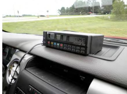
**Project Description:** This distance measuring instrument (DMI) uses a GPS receiver to measure pavement distances. The unit is self-calibrating, so it can be moved from vehicle to vehicle; it plugs into the vehicle's 12-volt electrical system.
