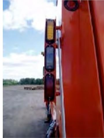
**Project Description:** The cost of the strobe light system currently used on MnDOT snowplows has been rising, and is now approximately \$300 more than a new LED warning light system. This project tested the effectiveness of this alternative to the higher-priced strobe lighting.
