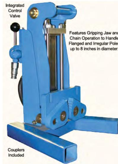
**Project Description:** The district's current practice of pulling sign posts with a crane boom sometimes results in the post breaking, which can be hazardous for the crew, the traveling public, the sign truck and the crane boom itself. The district will test an attachment to the crane boom—the REL-SPP hydraulic sign post puller, which features a gripping jaw and chain operation to handle flange and irregular poles up to 8 inches in diameter.
