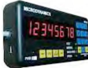
**Project Description:** Maintenance crews often need to measure distances along a roadway or between roadside features, such as when setting up traffic control. This vehicle-mounted unit measures distance using battery power or by plugging into a vehicle's 12-volt electrical system, so no hardwire connection is needed. The unit has an internal GPS module and stores distance, speed and GPS data for later retrieval.
