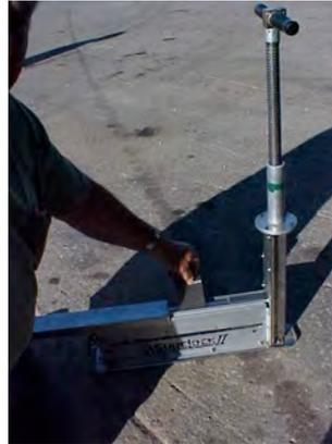
**Project Description:** Erosion blankets are used to help control soil erosion in and around roadside ditches, median ditches, slopes and culvert ends before rip-rap is placed. This staple gun is used to secure erosion blankets using 6-inch staples.
