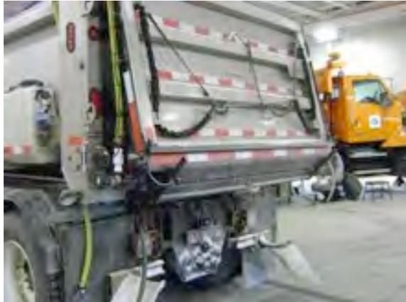
**Project Description:** The sander typically used on district tow plow trucks cannot raise its dump box high enough to use its entire load of material when pulling a tow plow or other trailers. Maintenance crews must also remove a sander mounted on a truck to allow the truck to be used for activities other than winter maintenance. The tailgate slurry sander resolves these issues by allowing full use of material and reducing the staff time needed to prepare trucks for operation in the field.
