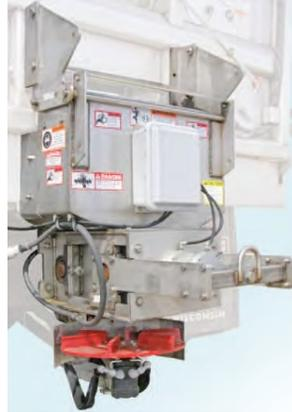
**Project Description:** Demonstrations have shown that applying salt as a slurry mixture reduces salt application rates and improves regain times. The Monroe RTS Replacement Tailgate Sander with roller mill slurry spreader can be used for this type of salt application. While the roller mill slurry spreader was developed for a live bottom V-box spreader, the spreader's manufacturer indicated that the unit can be used with the district's newer plow trucks that have elliptical boxes.
